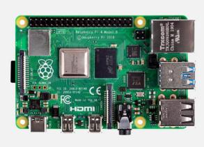
Raspberry Pi 4 Model B features a high-performance 64-bit quad-core processor, dual-display support at resolutions up to 4K via a pair of micro HDMI ports, hardware video decode at up to 4Kp60, up to 8GB of RAM, dual-band 2.4/5.0 GHz wireless LAN, Bluetooth 5.0, Gigabit Ethernet, USB 3.0, and PoE capability (via a separate PoE HAT add-on). For the end user, Raspberry Pi 4 Model B provides desktop performance comparable to entry-level x86 PC systems.
