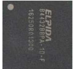
The markings on the new LPDDR2 device are clearly visible and read:<br>U1<br>ELPIDA<br>B443288PA-1D-F<br>16250R01300 |
