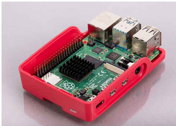
Figure 1. A Raspberry Pi in a case with a heatsink
