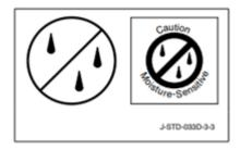
Although MSL1 does have floor life restrictions, an MSL1 product is not considered a moisture-sensitive product and therefore no MSID label should be present.
