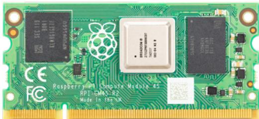
Raspberry Pi Compute Module 4 SODIMM (CM4S) is a System on Module (SoM) containing processor, memory, eMMC flash, and supporting power circuitry. These modules allow a designer to leverage the Raspberry Pi hardware and software stack in their own custom systems and form factors. The SODIMM form factor compute modules have 18 additional GPIO pins compared to the standard Raspberry Pi boards, for a total of 46, opening up more options for designers.
